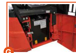
C Optional different battery capacities for different operation needs, optional Aquamatic battery self-filling system for easy battery maintenance.
